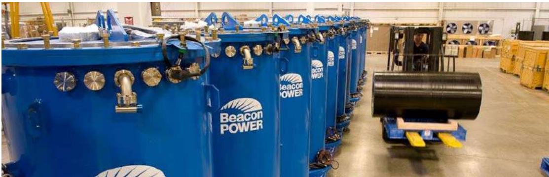
Figure 39: Photo of Beacon Power's flywheels [6]. The fiber composite flywheel itself is seen to the right on the fork-lift. Each unit is 100 kW. Photo from manufacturer's store.
