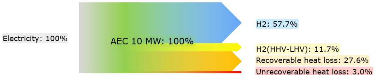
Figure 58: The energy inputs and outputs of an AEC (2020, 10 MW hydrogen plants). Data is derived from Ramboll references.
