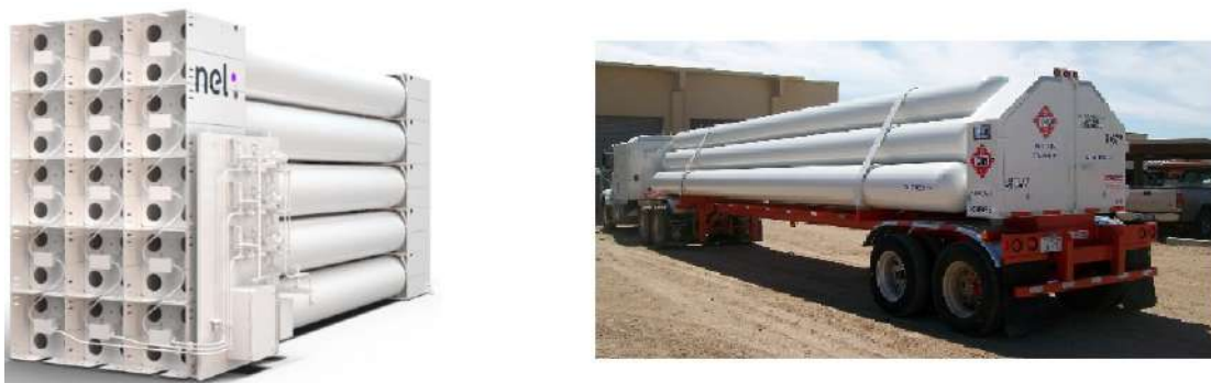
Figure 28: (left) Hydrogen storage of Type I steel tanks, (right) Hydrogen tube truck with Type I steel tanks [24], [25]
