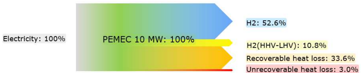
Figure 59: The energy inputs and outputs of a PEMEC (2020, 10 MW hydrogen plants). Data is derived from Ramboll references.
