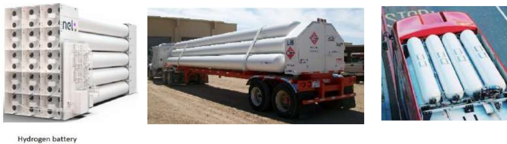
Figure 22: Hydrogen storage, transportation and fuel tank.
