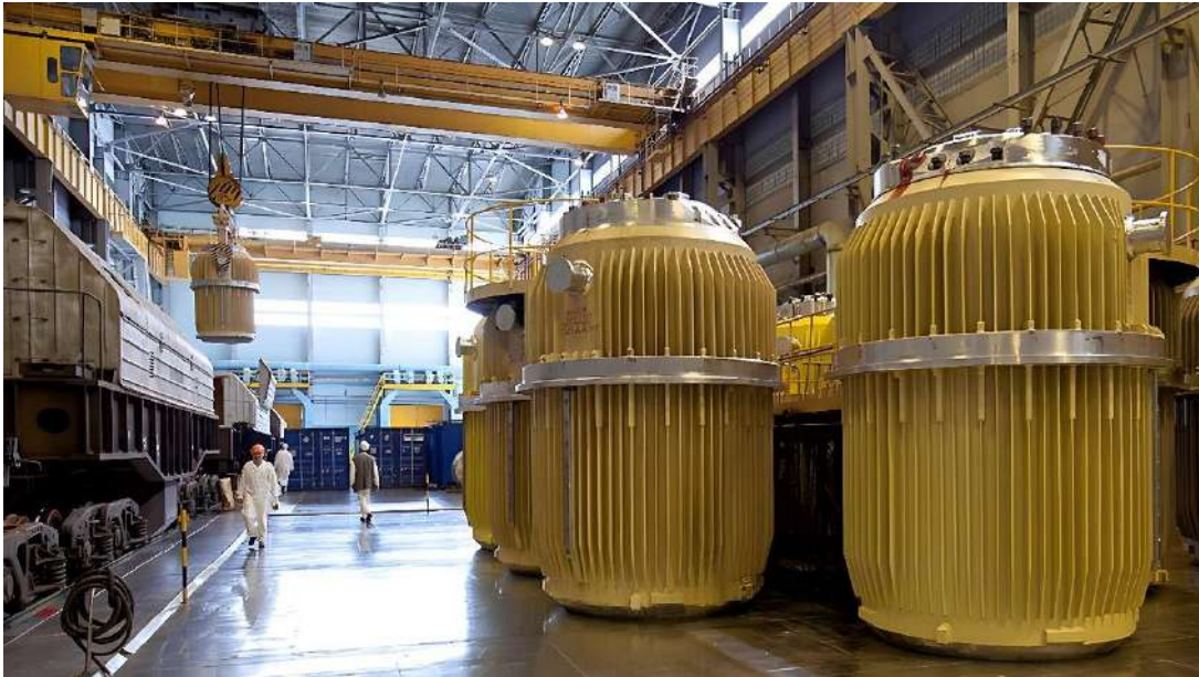
Figure 41: Unloading specialized containers from spent nuclear fuel transport railcars in Russia [3].
