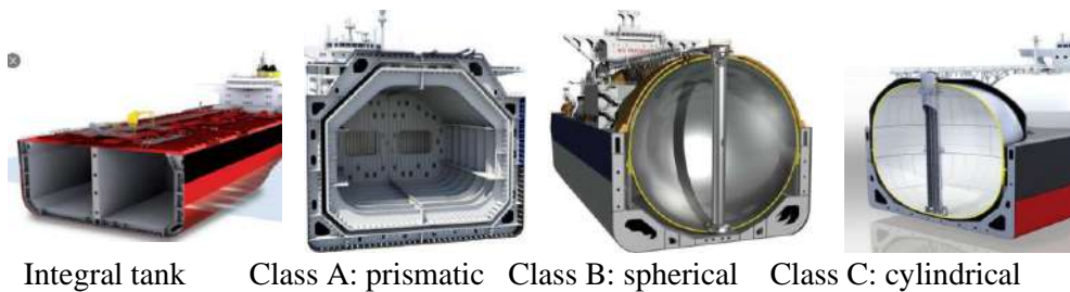
Figure 29: Different tank classes. The most cost-efficient onboard storage of ammonia seems to be class C (pressurized tanks) [3]
